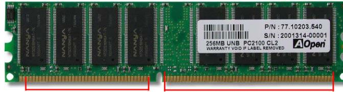
**Note:** Please pay attention to the Blue slots. To run dual channel speed, you should insert the RAM in the slot of DIMM A1 and DIMM B1 or DIMM A2 and DIMM B2. **Please don't use the different frequency DIMM on dual channel**
